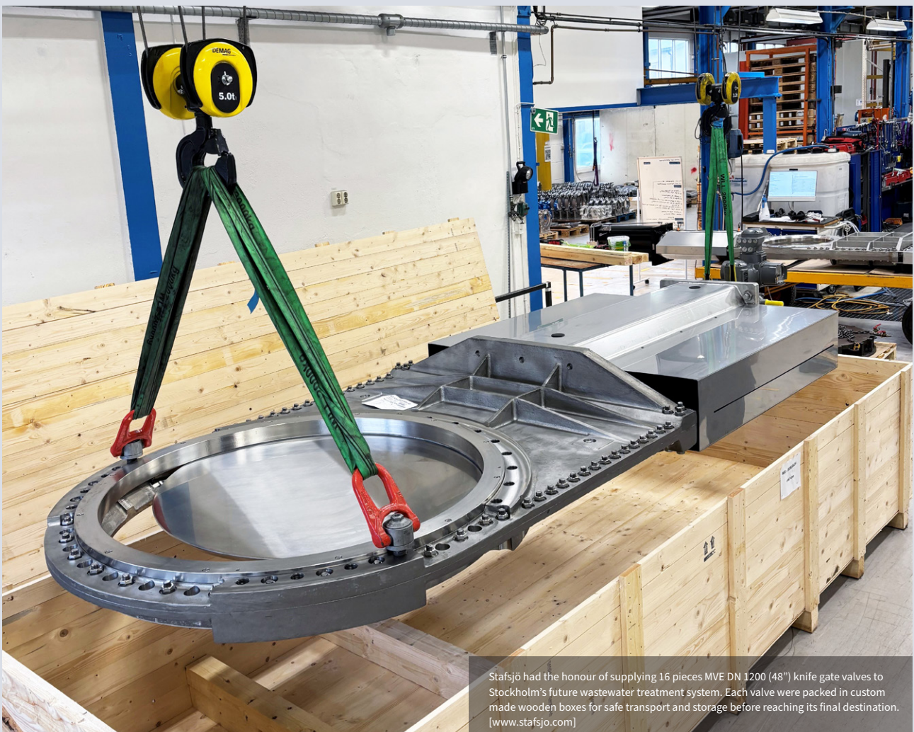
Before delivery, the Stafsjö's knife gate valves are subject for pressure tests with water in both open and closed position according to EN 12266-1:2003 rate A. No visually detectable leakage is allowed for duration of the test. [www.stafsjo.com]
