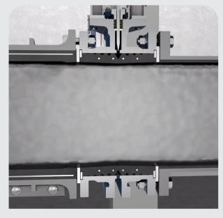
The full bore SLF form a rubber lined extension of the pipe system when it is opened position with no area for media build up.
