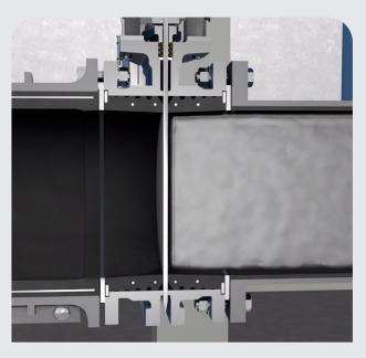
When the valve cycles to closed position the two seats are displaced axially forming a seal with the gate until it forms a complete closure -100% tight in any pressure direction.
