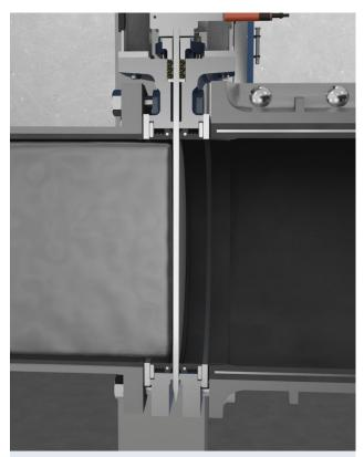
When the valve cycles to the closed position the two seats are displaced axially forming a tight seal with the gate through the entire stroke for 100 % bubble tight seal in all directions.
