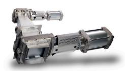
The Junk Trap (JT) is specially developed to minimize turbulence, erosive wear and build-up of solids and reject material. The JTV knife gate valve is installed in a slightly inclined position on the discharge side of reject tank to ensure a full release of media when opened and a tight shut-off when closed. Further information on the JT solution is available on www.stafsjo.com.
