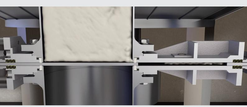
Pulp tower isolations require full bore and cavity free valves to assure a smooth pulp stock feed. It is crucial the valve ensure a safe and tight shut-off to avoid dewatering the pulp stock and at maintenance to guarantee the work can be performed safely on related process equipment. High pulp concentrations in the range 7 - 14 % are common and place special requirements on the knife gate valve. Stafsjö's HG has the technology to master the challenges.
