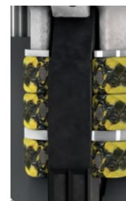
Box packing Optional top scraper TwinPack braids TwinPack braids Bottom scrapers TwinPack braids
