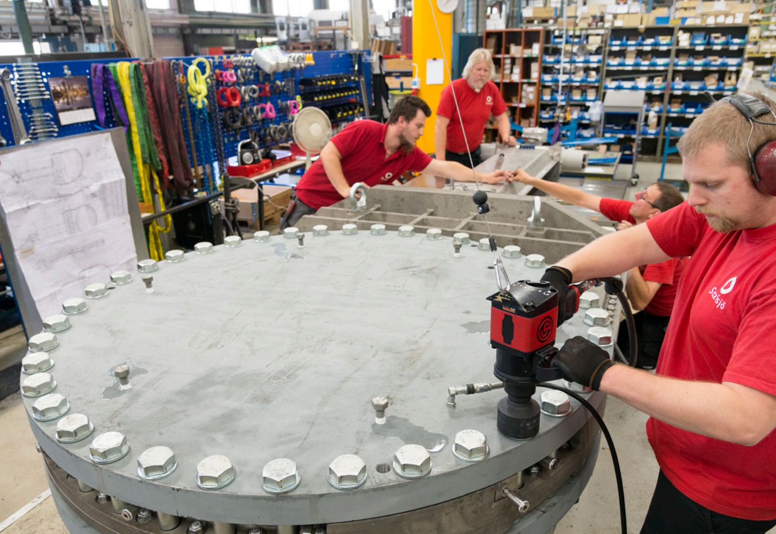
Assembling of the MV DN 1600 (64") at Stafsjö's workshop in Stavsjö, Sweden.
