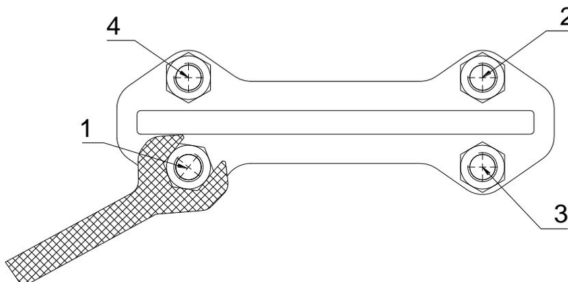
**Figure 5: Tighten gland nuts crosswise**
