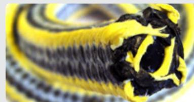
The TwinPack packing is strong and flexible. It is made up of braided PTFE fibers (black) and strong aramid fibers (yellow) in the corners to ensure excellent strength, wear and chemical resistance. The rubber core (black) keeps the packing compressed tightly against the gate.
